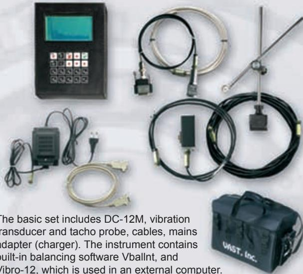
The basic set includes DC-12M, vibration transducer and tacho probe, cables, mains adapter (charger). The instrument contains built-in balancing software VbalInt, and Vibro-12, which is used in an external computer. A nylon carrying bag is furnished with the set.
